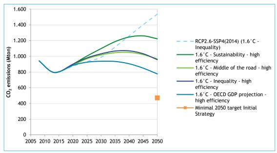
Figure 12 - CO<sub>2</sub> emission projections of shipping in four 1.6 °C High Efficiency scenarios
