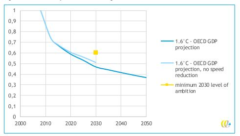
Figure 17 shows the development of the fleet-average AER. It could only be calculated for the scenario without speed reduction. Measured in this way, the carbon intensity improved by approximately 12% between 2008 and 2012 and is projected to improve by 33% by 2030. This would imply that the efficiency of international shipping has to improve by a further 7% to meet the 2030 level of ambition, which, in that case, would be beyond BAU.
