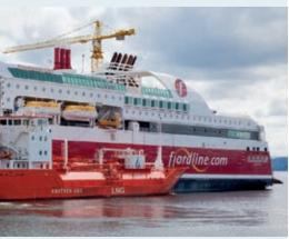
The gas-powered Ro/Ro passenger ferry Stavangerfjord being refuelled in Norway.
