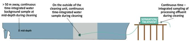
Figure 3: Schematic arrangement of sampling.
