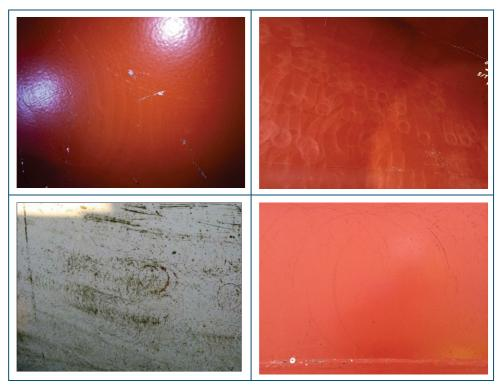
Figure 4: Examples of paint damages.
