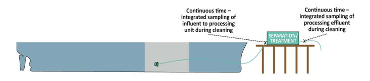
Figure 2: Schematic arrangement of sampling.
