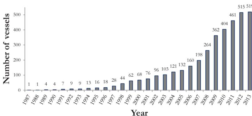
Figure 2: Number of various types of vessels with SCR
