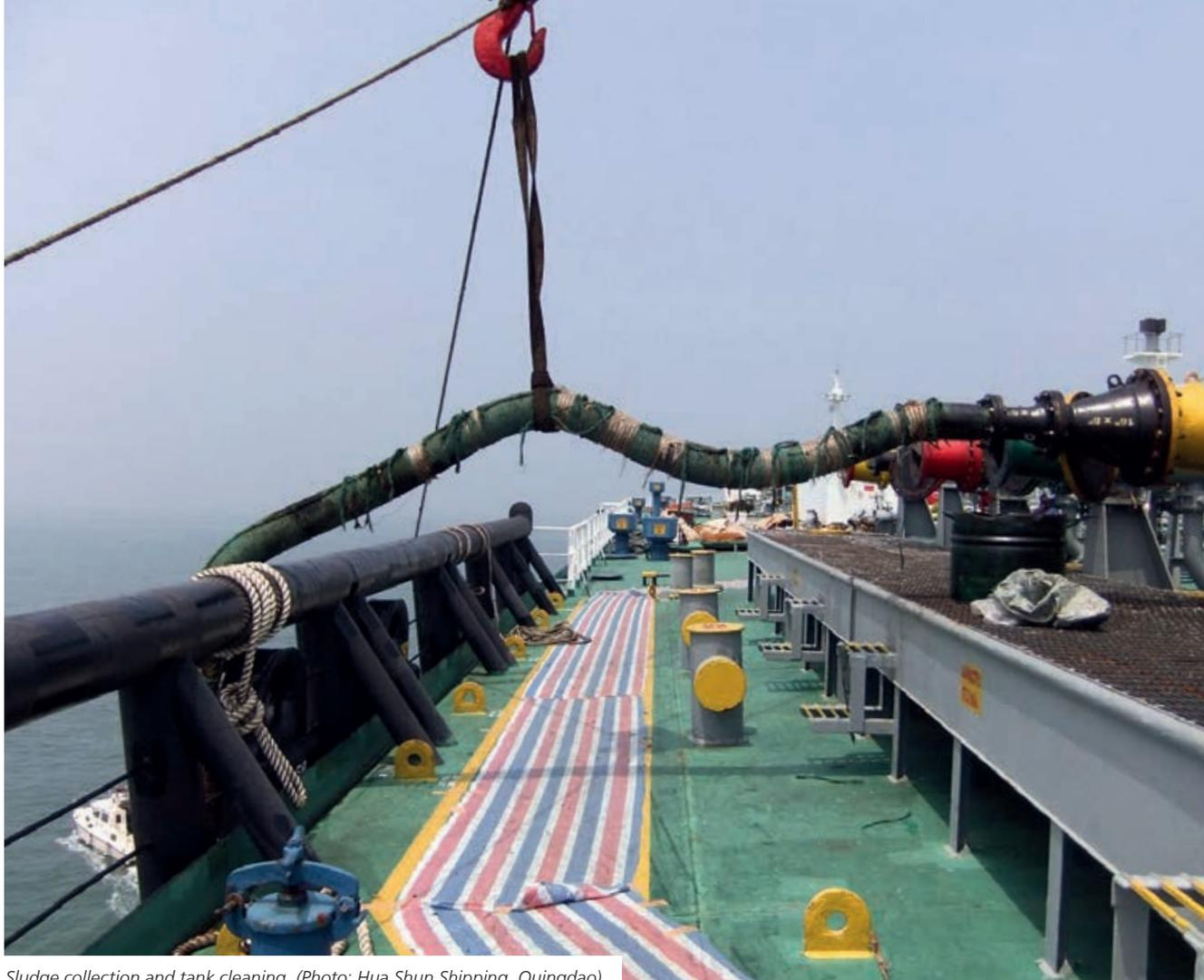
Sludge collection and tank cleaning. (Photo: Hua Shun Shipping, Qingdao)
