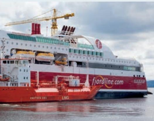
*The gas-powered Ro/Ro passenger ferry Stavangerfjord being refuelled in Norway.*
