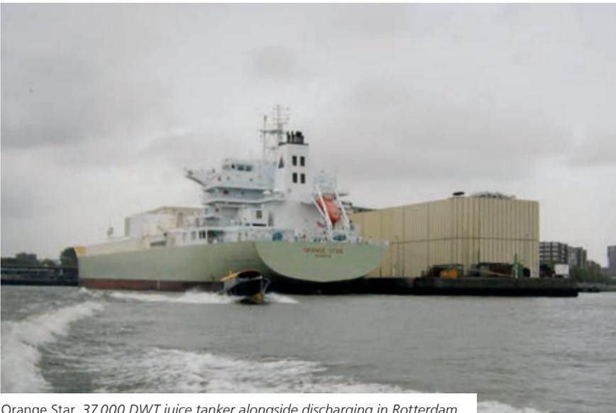
Orange Star, 37,000 DWT juice tanker alongside discharging in Rotterdam.
