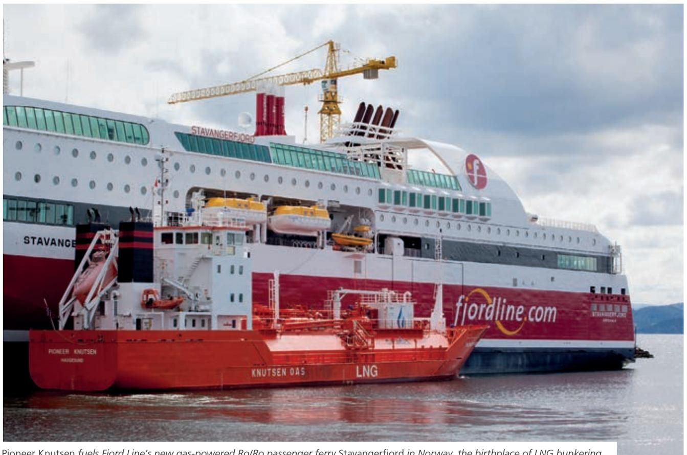
Pioneer Knutsen fuels Fjord Line's new gas-powered Ro/Ro passenger ferry Stavangerfjord in Norway, the birthplace of LNG bunkering.
